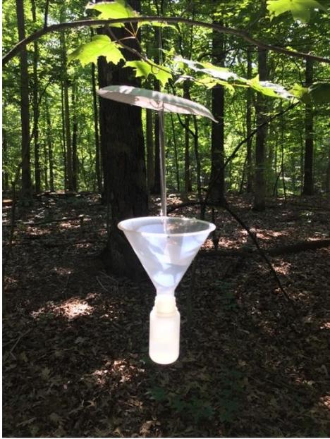
Figure 2. Window trap. Window traps are a flight interception trap. It has a plastic transparency sheet attaching to a funnel than a jar. When fly beetles hit the plastic sheet, they will drop into the funnel which lead them into the jar.
