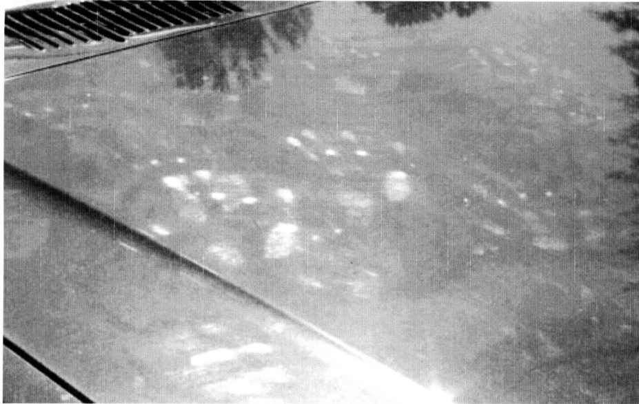
Figure 5: Three dimensional handprints of a polishing mitt scratch into the engine hood of a car as observed by Beaty (Beaty, 2003).
