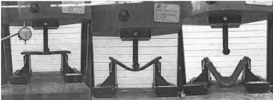
Figure 4- 3 Point-bend test being performed on SATEC
