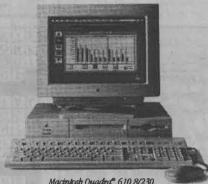
Macintosh Quadra® 610 8/230, internal AppleCD™ 300i CD-ROM Drive, Apple® Color Plus 14" Display, Apple Extended Keyboard II and mouse.
