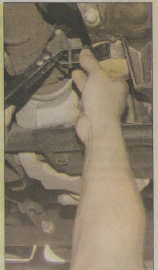
You may need an oil filter wrench to break the seal on the old filter.
