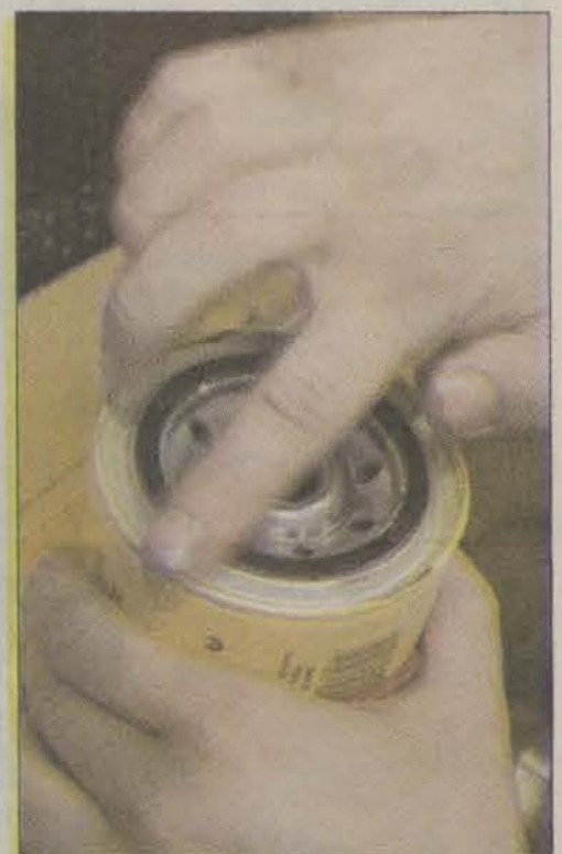
Make sure that you coat the gasket of the new oil filter with some of the used oil so next time you change your filter it comes off easily.
