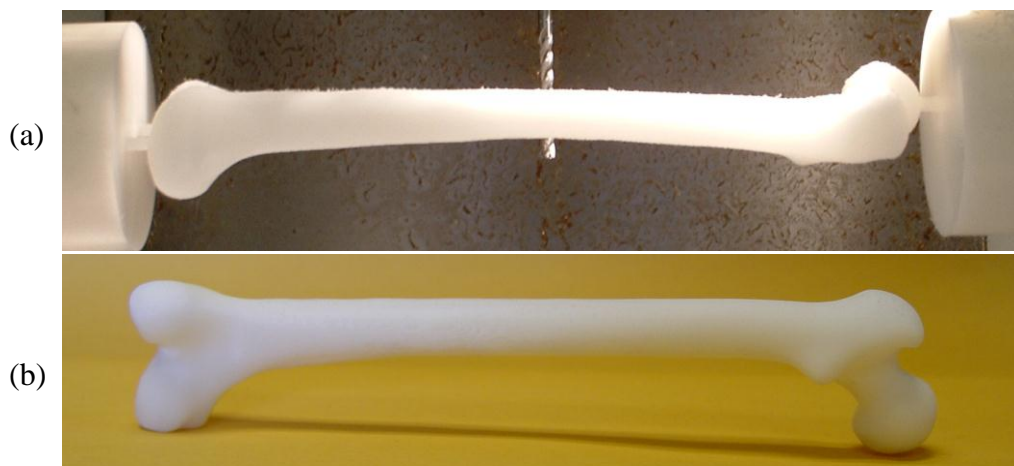
Figure 17 - Femur bone model; (a) with supports, (b) finished
