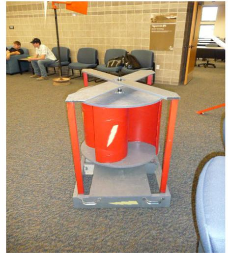
generally less than 1. Figure 1 shows a student built Savonius wind turbine.
