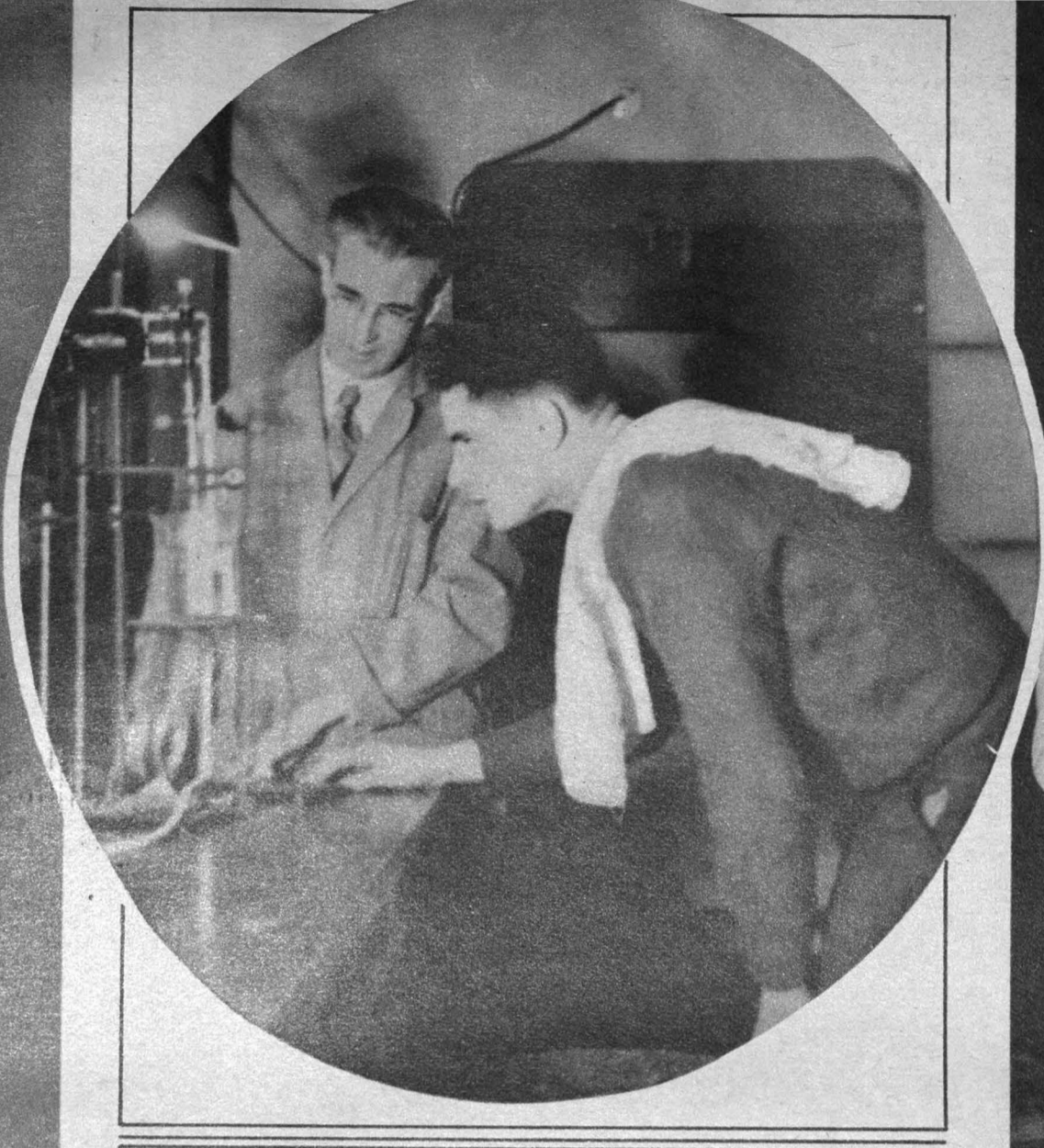
A N ALLOY WHICH MELTS AT 47 degrees centigrade has been developed at Colgate University by Dr. Sidney J. French and Donald J. Saunders. The new alloy contains lead, tin, cadmium, bismuth and indium.
